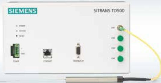
Up to 192 measuring points enable continuous temperature profiles to be determined in the smallest possible space.
