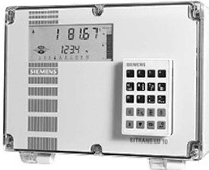
Using the patented Sonic Intelligence echo-processing software to measure level, space, distance, volume, or average/differential, the LU10 provides superior reliability and accurate measurement in vessels up to 60 meters in height (200 ft). Furthermore, transducers can be mounted up to 365 meters (1200 ft) from the monitor. Readings are displayed in user-selectable linear engineering units on the backlit LCD.
