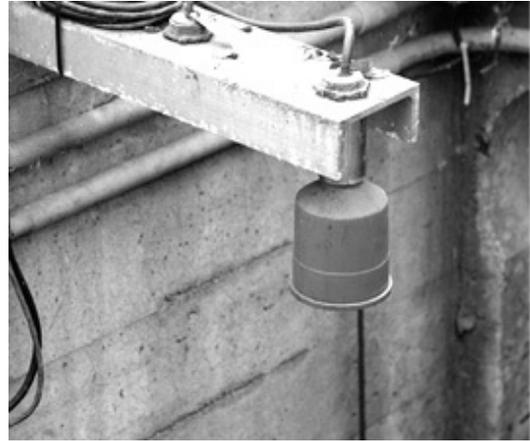
Ultrasonic level measurement instrumentation offers non-contacting technology that is virtually maintenance free and cost effective in many applications, from the water and wastewater industries to solids and liquids measurement in a variety of industrial settings.
