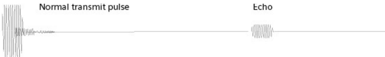
This signal is digitized by the transceiver's A/D converter and changed into an echo profile, which is a measurement of the echo energy versus time.
