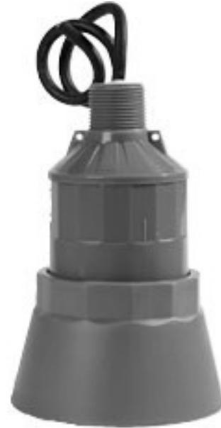
When installing a submergence shield, ensure it is properly seated and even across the transducer. Check for leaks by placing the assembled unit in a bucket of water and see if any bubbles leak out. Leaks indicate the shield has not been pulled down far enough to properly seat the pressure clips.
